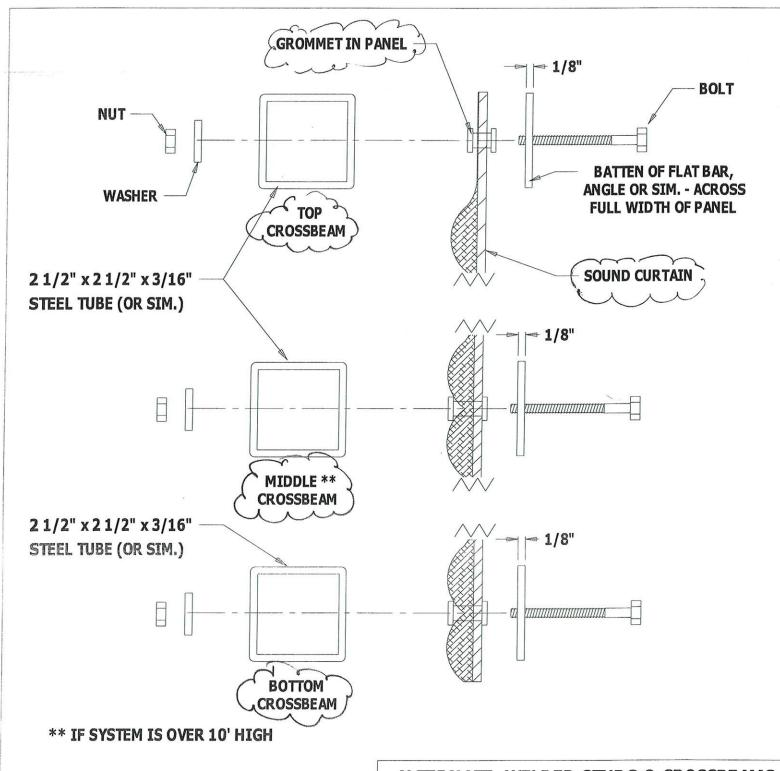
NOTE: SIZING AND SPACING OF VERTICAL COLUMNS OR POSTS TO BE DETERMINED BY STRUCTURAL ENGINEER.
